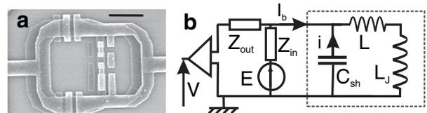
FIG. 1. (a) SEM picture of the sample. The flux qubit is the small loop containing four Josephson junctions in a row; the SQUID is constituted by the outer loop containing the two large junctions. The bar equals 1  $\mu$ m. (b) Measuring circuit diagram. The SQUID, represented by its Josephson inductance  $L_J$ , is shunted by an on-chip capacitor  $C_{sh}$  through superconducting lines of inductance  $L$ , forming the plasma mode.
